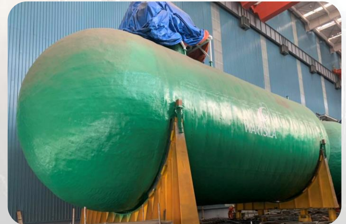
LTC on Whole Tank Insulation
